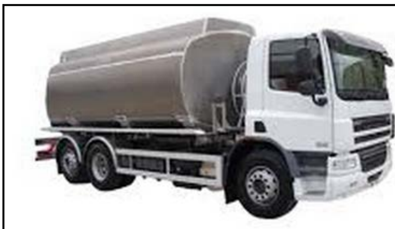
Plate 14.2.7 Example of a 7m Road Tanker with 9 cubic metre capacity
