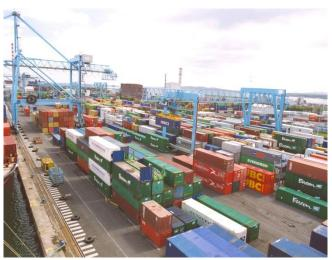
Containers are moved between the stacks and the quay side cranes by special heavy duty truck and trailer combinations or by reach stackers.
